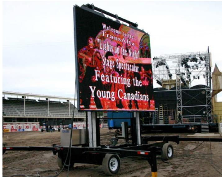
Custom trailers transport 12.5-foot-tall by 16.7-foot-wide LED screens to and from each event at the Calgary Stampede rodeo and entertainment show in Calgary, Canada. Each mobile LED screen consists of 25 Lighthouse Technologies LH 1650D LED panels.
